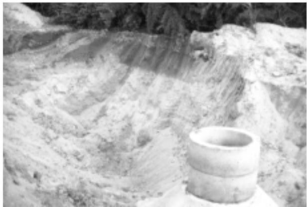
Glaciofluvial deposits typical of the study area. Exposure is in an excavation immediately south of the Harbor Hill moraine near the DeFriest Blowout. Note the wide range of particle sizes.
